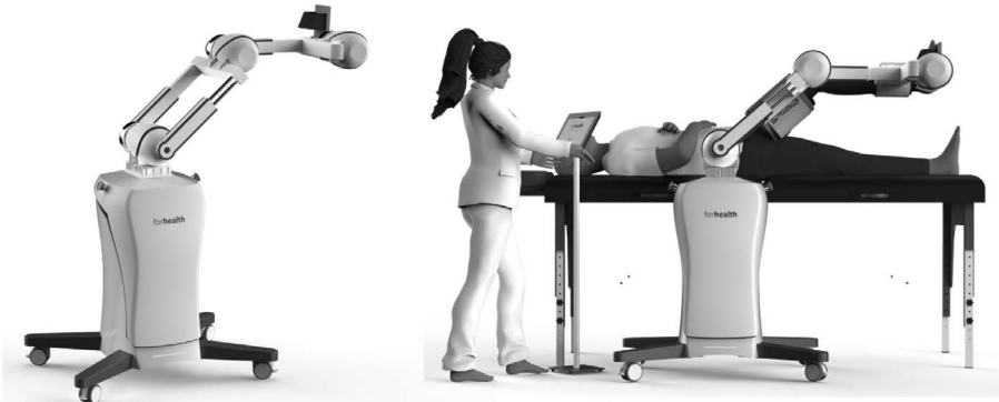
FIGURE 14.7 Rehub Buddy, the Intelligent Lower Limb Orthosis.
